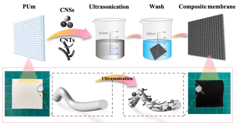
Fig. 3-4. Schematic demonstration for the preparation of PU composite membranes.
