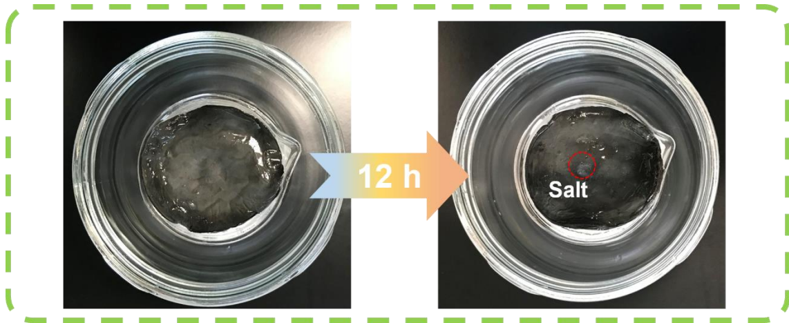
Fig. 4-27. The photos of GZPS device system before and after 12 h solar irradiation.
