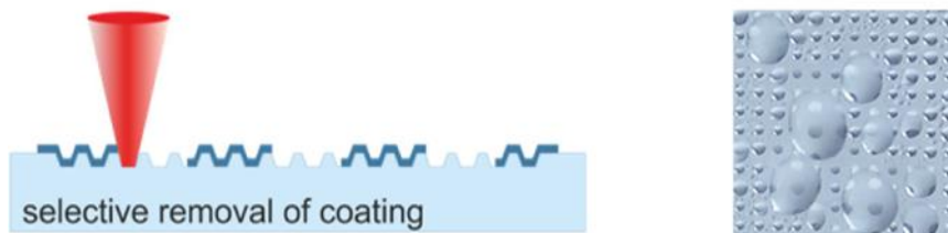
Fig. 1-5. Steps in the production of (a) superhydrophilic surfaces through fs-Laser structuring, (b) superhydrophobic surfaces via the deposition of a Teflon-like polymer layer, and (c) high-contrast micropatterns through selective laser ablation. Reproduced with permission from ref [30] Copyright © 2018, American Chemical Society.
