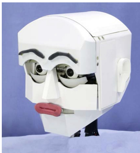
Fig. 5-1 Head of bipedal walking humanoid robot "KOBIAN".
