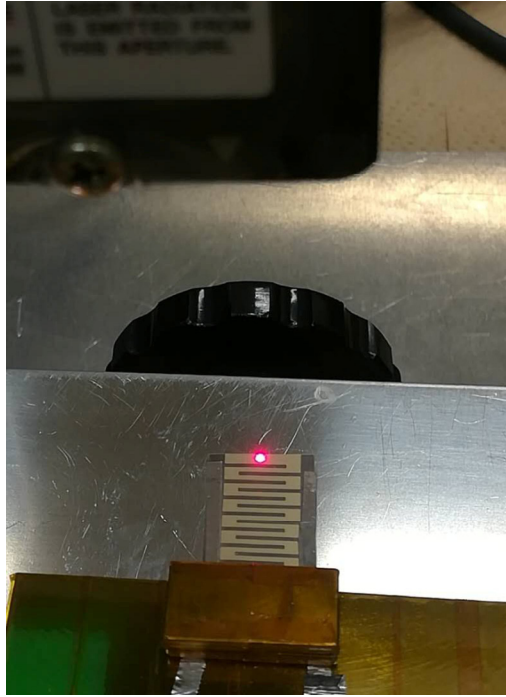
Figure 6-2. Bending displacement measurement system.
