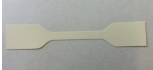
Figure 5-1. A dumbbell specimen for tensile testing (JIS K-6251-7)
