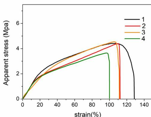
**Figure 7-8.** Stress–strain curves of polycaprolactone nanofiber tubes with two layers (1), three layers (2), five layers (3), and ten layers (4) prepared by thermal treatment at 50 °C.
