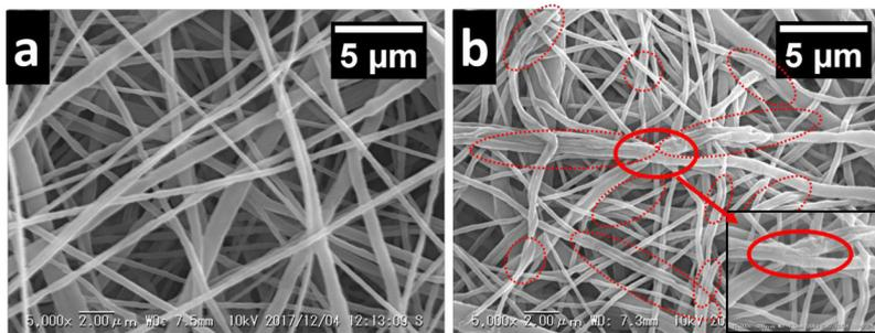
**Figure 7-4.** Scanning electron microscopy images of polycaprolactone nanofibers (a) before and (b) after thermal treatment at 50 °C.
