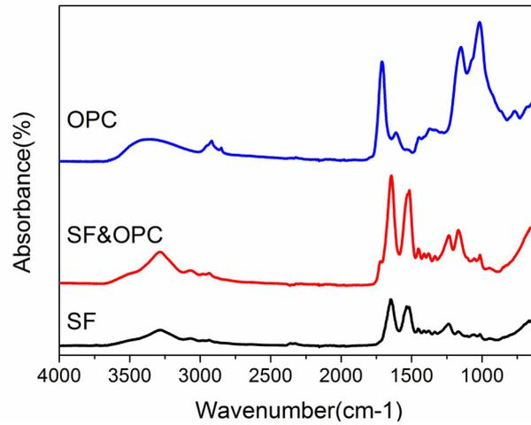
**Figure 5-4.** FTIR spectra of OPC powder, SF nanofiber and SF & OPC nanofibers.
