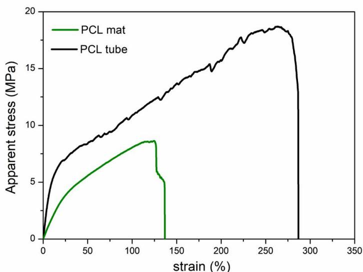
**Figure 4-3.** Stress–strain curves of polycaprolactone nanofiber tube with two layers and polycaprolactone nanofiber mat by thermal treatment.
