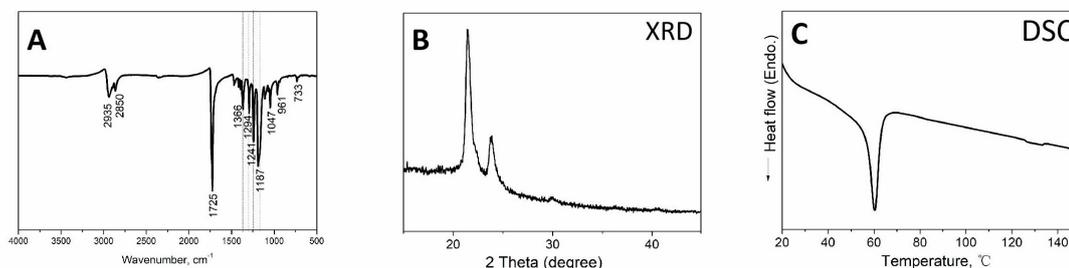
**Figure 7-6.** (A) Fourier-transform infrared spectrum of a PCL nanofiber mat. (B) X-ray diffraction pattern of a PCL nanofiber mat. (C) Differential scanning calorimetry thermogram of PCL nanofibers.
