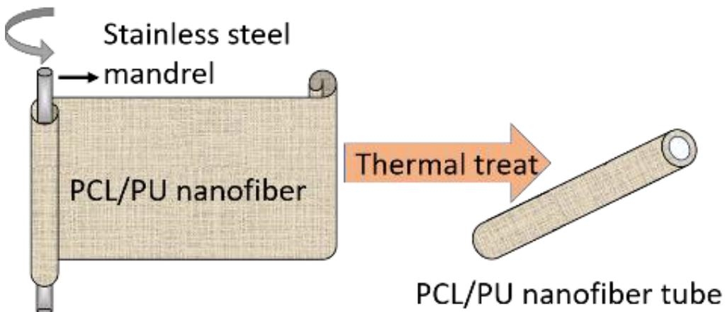
**Figure 6-3.** Polycaprolactone–polyurethane (PCL–PU) nanofiber tube preparation.
