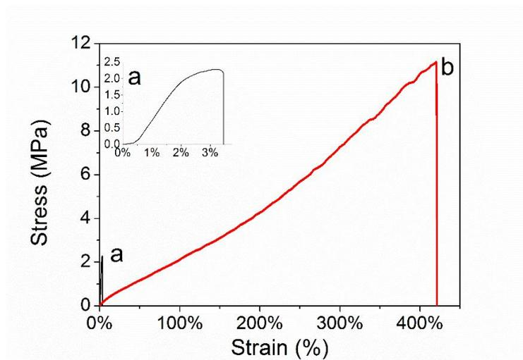
**Figure 5-3.** Stress–strain curves of the prepared (a) SF nanofiber, (b) PU nanofiber.
