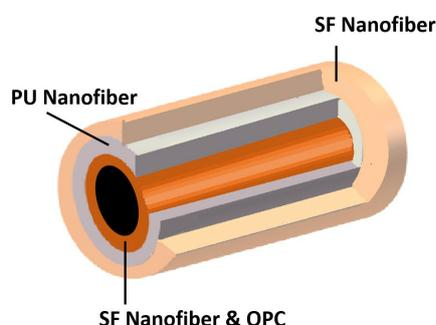
**Figure 5-1.** Schematic illustration of a three-layer nanofibrous tube
