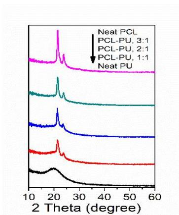
**Figure 6-8.** X-ray diffraction patterns of nanofiber mats fabricated from polycaprolactone (PCL), polyurethane (PU), and their blends (PCL–PU)
