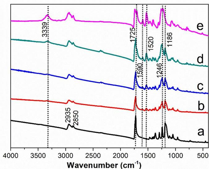
**Figure 6-9.** Fourier-transform infrared spectra of nanofiber mats fabricated from polycaprolactone (PCL), polyurethane (PU), and their blends (PCL–PU). a, PCL, b, PCL–PU 3:1, c, PCL–PU 2:1, d, PCL–PU 1:1, and e, PU
