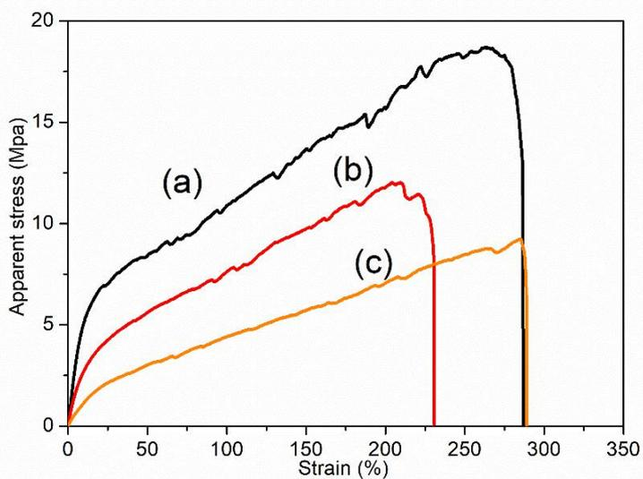
**Figure 6-10.** Stress–strain curves of polycaprolactone–polyurethane (PCL–PU) nanofiber tubes thermally treated at 50 °C. a, PCL–PU 3:1, b, PCL–PU 2:1, and c, PCL–PU 1:1
