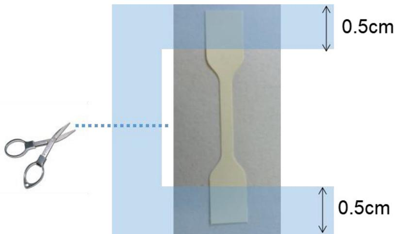
**Figure 4-1.** A dumbbell specimen for tensile testing (JIS K-6251-7)
