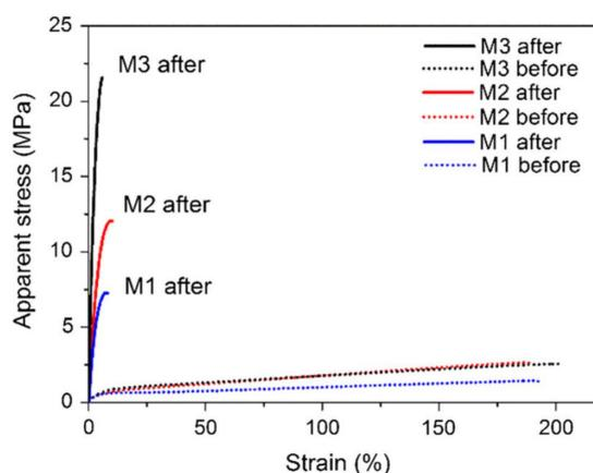
**Figure 3-11.** Stress–strain curves of the prepared membranes before and after treatment.
