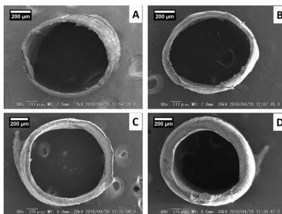
**Figure 7-5.** Scanning electron microscopy images of polycaprolactone nanofiber tubes with (A) two layers, (B) three layers, (C) five layers, and (D) ten layers prepared by thermal treatment at 50 °C.
