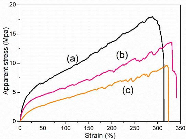
**Figure 6-11.** Stress–strain curves of polycaprolactone–polyurethane (PCL–PU) nanofiber tubes thermally treated at 60 °C. a, PCL–PU 3:1, b, PCL–PU 2:1, and c, PCL–PU 1:1
