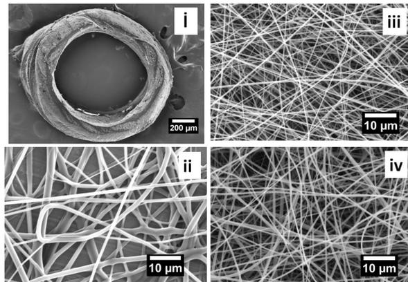
**Figure 5-2.** SEM images of (i) nanofiber tube (ii) PU nanofibr (iii) SF nanofibers (iv) SF & OPC nanofibers.
