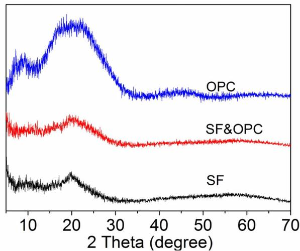
**Figure 5-5.** XRD spectra of OPC powder, SF nanofiber and SF & OPC nanofibers
