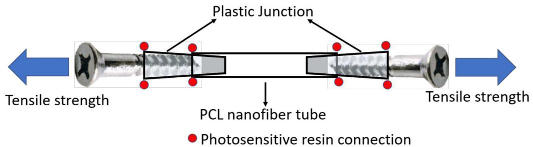
**Figure 4-2.** Schematic of a nanofiber tube specimen used for tensile testing
