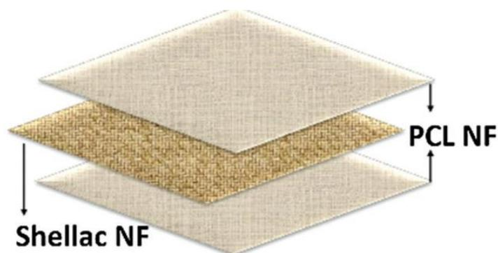
**Figure 3-4.** Schematic illustration of a PCL/shellac/PCL sandwich structured membrane.
