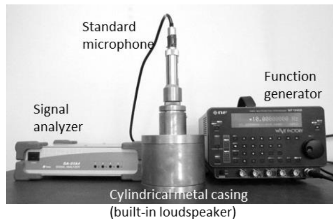
Fig. 3-5 Micro-hole inspection system. The inspection system consists of a cylindrical inspection container, a signal analyzer(SA-01A4, RION Co. Ltd) and a function generator (WF1946B, NF Co. Ltd). Loud speaker is installed inside the metal inspection container. The cylindrical inspection container is about 150 mm in height.
