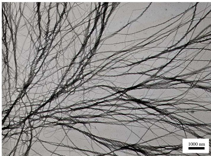
Figure 4. TEM image of acetonitrile gel formed by gelator **3**.
