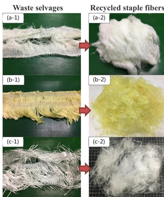
Figure 2.1 Recycled selvage and staple fibers. a-1) The left column shows the recycled Nomex®,(b-1) Kevlar®, and (c-1) PET selvage. The right column shows the (a-2) Nomex®, (b-2) Kevlar®, and (c-2) PET staple fibers.
