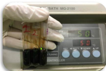
Figure 5-1. Dip-coating AP solution in PHBH monofilament at 50°C.
