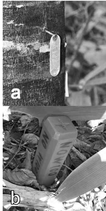
Fig. 3. (a) An aluminum plate holding the trunk ID number (Racetrack Aluminum Tags, Forestry Supplies Inc.) with a stainless steel nail (#12 \times 50mm) and (b) a red plastic pile (Etapron K-50, Juzen Corp.), driven into the ground at intervals of 10m, showing the coordinates (N[x]-W[y] axis) written with the oil-based marker; Magic Ink, Teranishi Chemical Industry Co., Ltd.) for the position in a 1-ha permanent plot for the Monitoring Sites 1000 Project in Kayanodaira.
