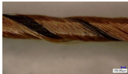
図8 An example of double PBO filament covered carbon fiber bundle (DCCF)
