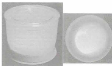
図 2 MILLIFLEX 100 FILTRATION FUNNEL (濾過ユニット) (0.45 μm membrane filter)
